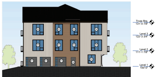
② Building Type 1 - 25 Units - East Elevation 3/32" = 1'-0"
