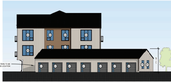
④ Building Type 3 - 25 Units - South Elevation 3/32" = 1'-0"
