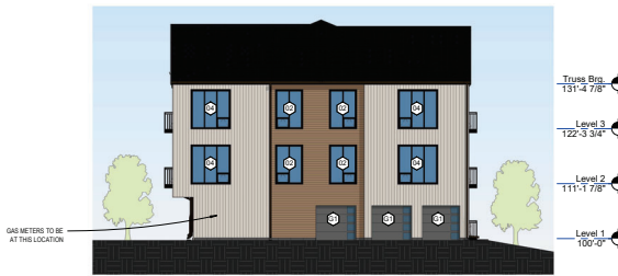
③ Building Type 1 - 25 Units - West Elevation 3/32" = 1'-0"
