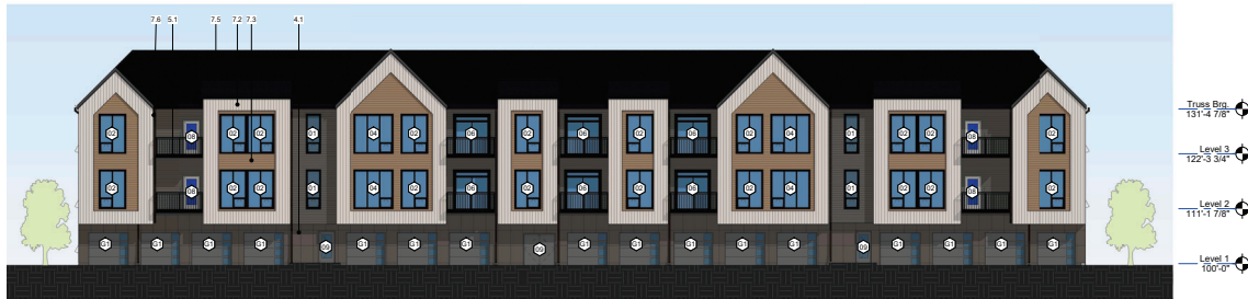
① Building Type 1 - 25 Units - North Elevation 3/32" = 1'-0"
