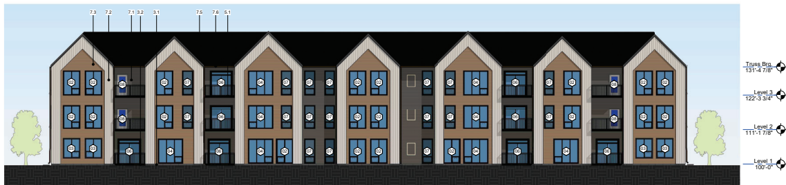
④ Building Type 1 - 25 Units - South Elevation 3/32" = 1'-0"
